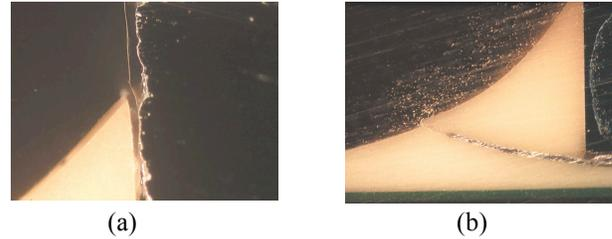
Figure 12. Underfill fillet delamination and crack
