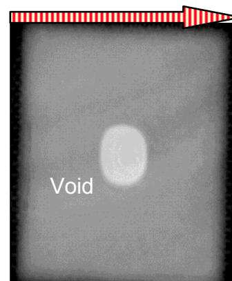
**Figure 6 : Typical one pass dispense results for underfill D**
