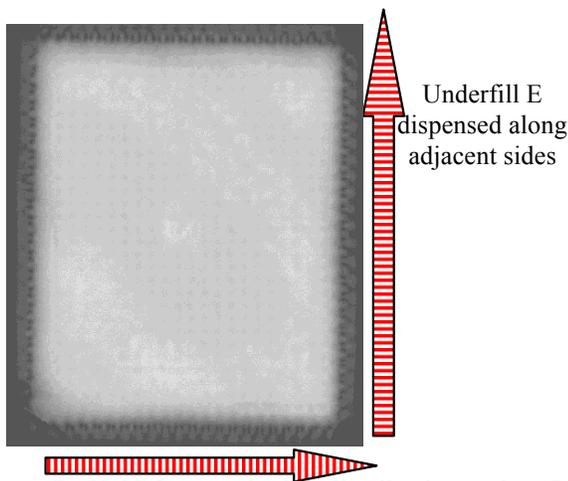
**Figure 7: Void-free underfill distribution using L-pass dispense method**
