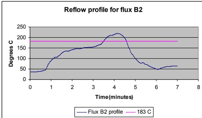
**Figure 4: Reflow profile for flux B2**
