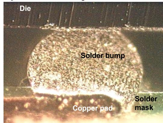
**Figure 13: Solder joint in PSGA-CSP assembled using treatment combination 19 placement parameters**
