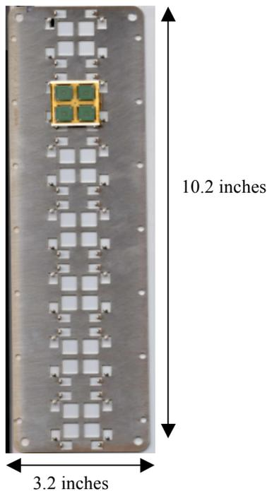
**Figure 2: Commercial PSGA-CSP placement fixture**
