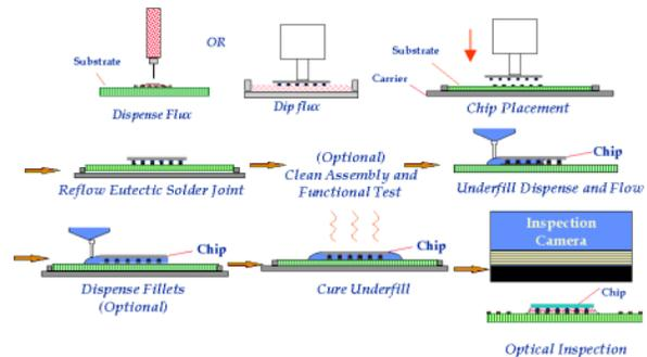
**Figure 9: Conventional flip chip assembly process**
