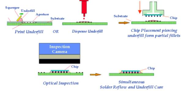
**Figure 8: Low cost-next generation flip chip assembly process**
