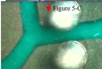
**Figure 5: Post-shear images for PSGA-CSP module assembled using dip flux A7**
