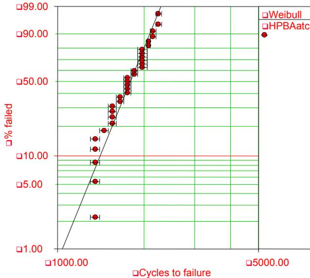
**Figure 12: Weibull distribution plot of air-air thermal cycle reliability results for PSGA-CSP packages using high performance underfill D and flux A7**
