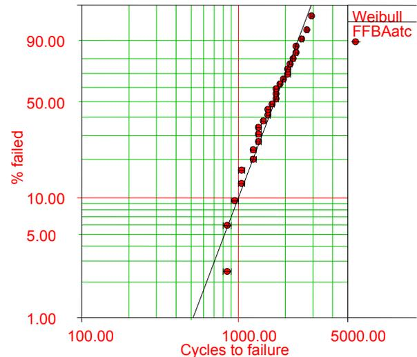
**Figure 11: Weibull distribution plot of air-air thermal cycle reliability results for PSGA-CSP packages using fast-flow snap cure underfill D and flux A7**
